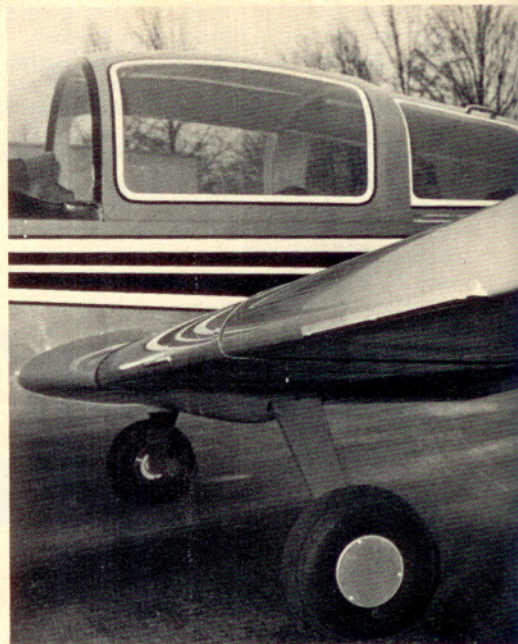
Inboard and outboard spoiler strips on the airfoil help make the Traveler slow to stall.
